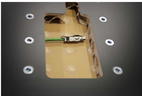
Fig. 5: Blind rivet nuts in lisocore® as fixing points for table legs
